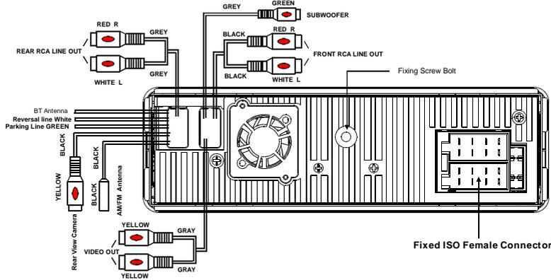
Note: 1. Parking wire must be connected, and the parking brake must be engaged in order for the monitor to work
