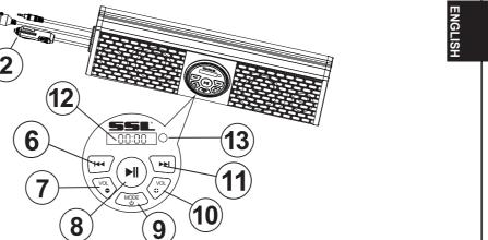
1)Power on the SB18 by plugging in the male cigarette lighter adaptor into (2) a 2) Press the button (9). The SB18 will automatically go in to arbitrary pattern
