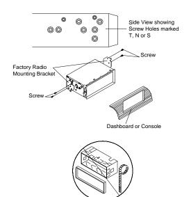
To fasten the unit to the factory radio mounting brackets.
