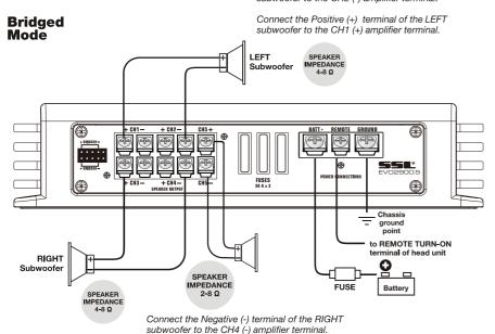
Connect the Positive (+) terminal of the RIGHT subwoofer to the CH3 (+) amplifier terminal.
