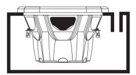
Box is given as internal air volume including driver displacement
